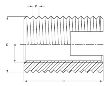
Female thread A = M16 Length B = 22 Male thread E = 20.0 Min hole depth blind hole = 27
